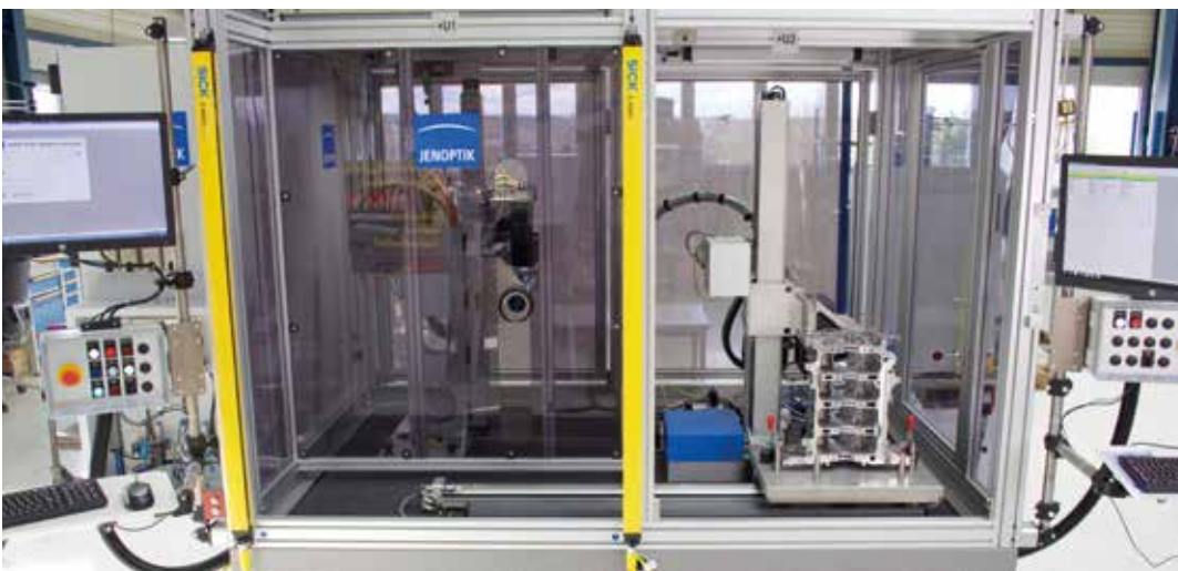
Combined cylinder inspection using B100 and CF1250
