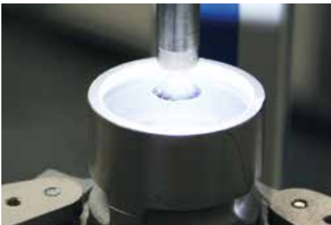
Inspecting inside bores
