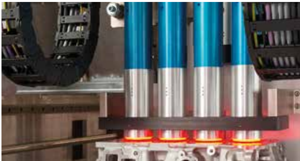
Simultaneous inspection in four cylinder bores using four B100 sensors
