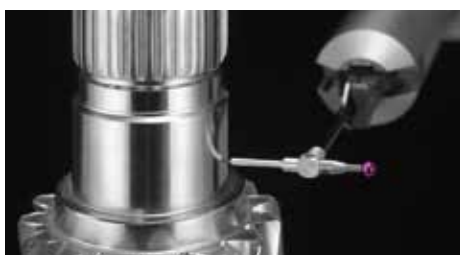
Twist measurement with a roughness stylus tip
