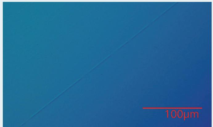
Comparison of optical surfaces without (left) and with (right) DLC after Windscreen-Wiper-Test
