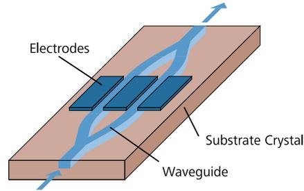
Schematic layout of an integrated-optical amplitude modulator
