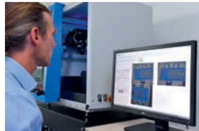
During the automatic scan process a 3D model is precisely composed using various views without reference marks. This innovation impressed the Jenoptik Innovation Workshop jury.
